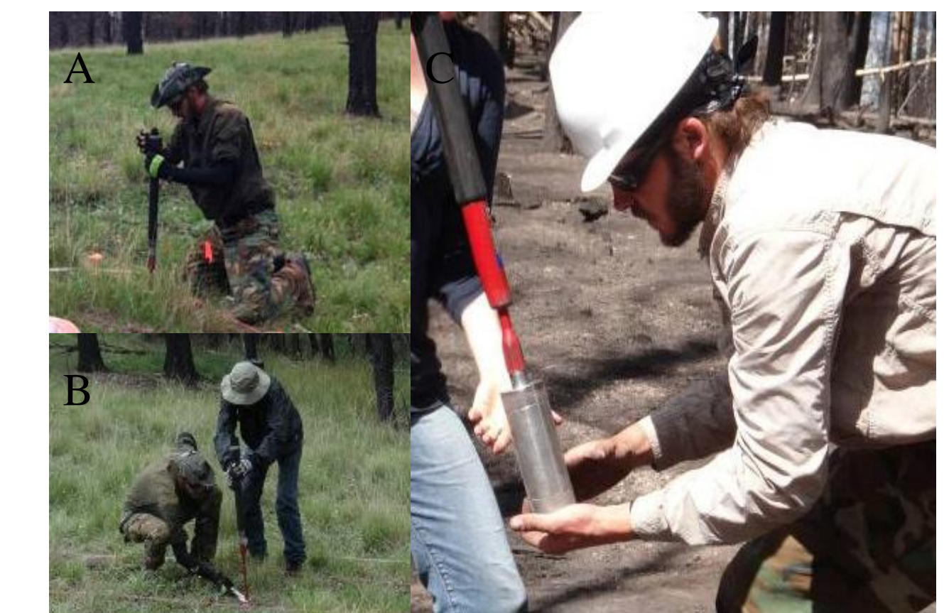
Figure 6. Soil coring process. A) Taking samples with the soil corer and slide hammer, B) removing soil core sample from ground with the aid of a wrench to minimize disturbance to surrounding soil, and C) removing soil core sample from slide hammer.
